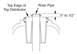
**Note:** Resin tank height can vary somewhat within manufacturing tolerance. So that the bottom distributor riser pipe has proper clearance with inside valve porting, check for the correct length, as shown above. Cut the riser pipe if needed to adjust the length. Be sure to remove burrs and sharp edges.
